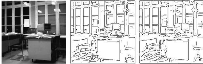
Fig. 5. (Left) Original image. (Center) Detection by Shen and Castan filter ( $s = 0.4$ ). (Right) Detection by Gaussian (derivative) filter ( $\sigma = 2.2$ ). Same SNR, Threshold = 2. The last image presents clearly edge delocalization.
