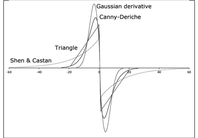
Fig. 3. Impulse responses of derivative filters used to compare localization properties. Filter scale parameters have been chosen to keep the same non-detection limit ( $d = 10$ ) under additive influence.
