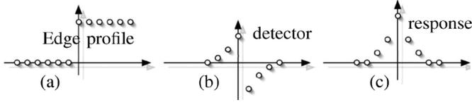
Fig. 2. (a) Discrete signal with one step. (b) Regularized derivative estimator. (c) Estimate of the derivative (denoted also as  $h$ ).
