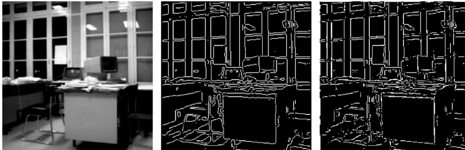
Fig. 8 From left to right: original image; image segmented in the classical way (CW); image obtained by our system (CC) with parameters \{d^p, d^l, l_{0,0}^p\} , p=0 , modulus approximation of the gradient, and real-world training image.
