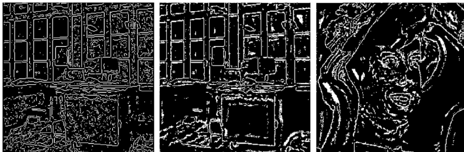
Fig. 14 Results on noisy (Gaussian noise of standard deviation 22) real images for identical ND and P . From left to right: segmented image by thresholding (upper threshold=17), segmented image by merging system. These two images are represented by approximately the same point on the curves of Fig. 13: ND \approx 27, P \approx 70 . The third image results from the merging of the image "Woman." (See original image "Woman" in Fig. 16.)
