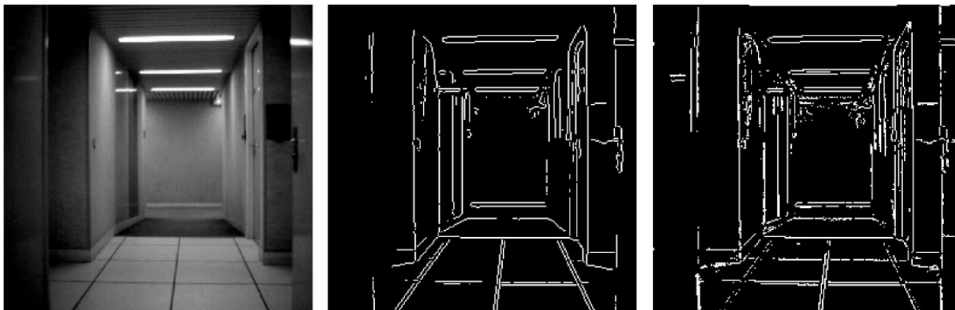
Fig. 11 From left to right: original image; image segmented by extraction of local maxima and hysteresis thresholding (upper threshold=20); image segmented by the classifier. The training has produced 86 polytopes.
