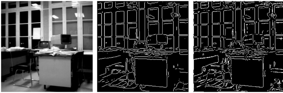
Fig. 10 From left to right: original image; image segmented by extraction of local maxima and hysteresis thresholding (upper threshold=20); image segmented by the classifier. The training has produced 86 polytopes.
